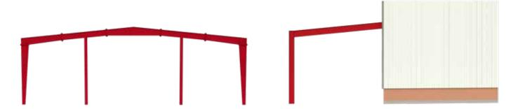
MULTISPAN MS-2 buildings have a gable roof with vertical sidewalls and end walls. Interior bay frames are rigid frames. The designation MS-2 implies two interior columns, and so on.
