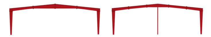
**CLEAR SPAN** buildings have a gable roof with vertical sidewalls and end walls. Interior bay frames are clear span rigid frames (without interior columns).
