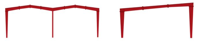
**MULTIGABLE** buildings have a roof with 2 or more gables, vertical sidewalls and vertical end walls. Interior bay frames are rigid frames.
